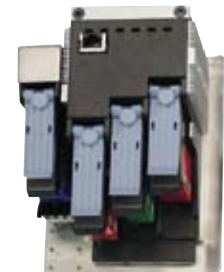
Fourth print cartridge added for full two-inch print area
