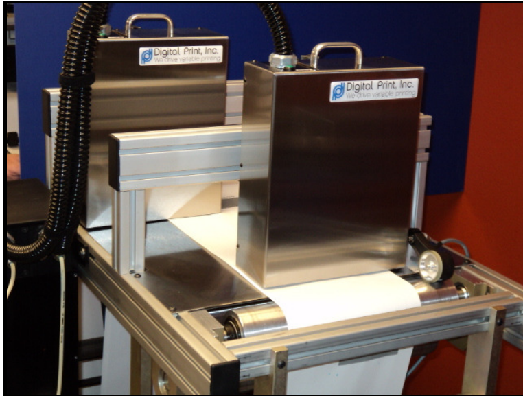
Two 5" DOD HAWK Print Heads on a web press mount
